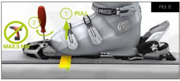
Adjust the AFD with the screw on the top so that the tester is still moveable but with a slight resistance. In this case, you reached a gap of 0.5 mm between AFD and the boot (Pict. 7).
