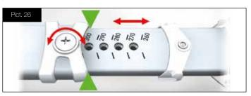
Close the ascender lock and slide the binding into the closed position in all versions.
