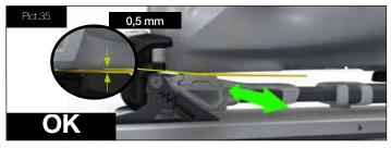
If the tester is not moveable, the gap is smaller than 0,5 mm, if you feel no resistance the gap is more than 0.5 mm. In both cases you need to re-adjust the AFS.
