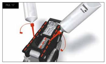
After finishing the heel lubrication slide on the heel and lock it in its original position.
