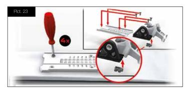
Insert the screw in the bottom side of the heel unit, and slide the whole unit to the closest mounting position on demo track and fix it with the screw.
