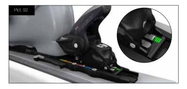
**NOTE:** If the forward pressure is not correct, readjust the boot sole length and check the SINGLE CODE. Please make sure that no boot is placed in the binding during adjusting!
