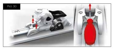
Take the Ambition brake arm, press it together and clap the brake pedal to a horizontal position. First click right then left side into place.
