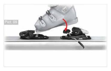
Check the elasticity and retention of the toe by pushing the boot inward and outward. The binding must re-center the boot easily and quickly from a 15mm lateral displacement (EL 7.5 AC Shift, EL 4.5 AC Shift - 10mm).
