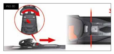
Now hook the brake into the heel housing.
