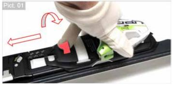
Slide the toe towards tail. At certain point the toe will stop, then release the laver and push it into the end position.
