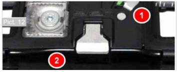
Finally, check the forward pressure, by placing a boot into the binding. If you have followed all steps correctly, the indicator should rest in the marked area.
