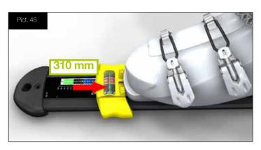
Go on with placing the toe track over the holes and fasten all screws in a cross pattern.
