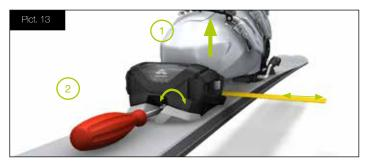
Adjust the AFD with the screw in the front so that the tester is still moveable but with a slight resistance. In this case, you reached a gap of 0.5 mm between AFD and the boot (Pict. 14).
