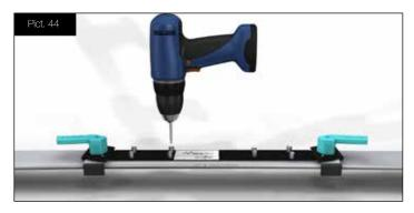
After drilling place a drop of glue into the holes. It lubricates the screws and seals the holes.
