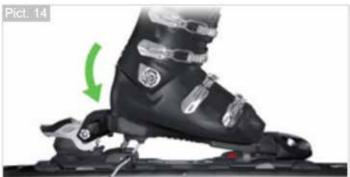
Check the elasticity and retention of the toe by pushing the boot inward and outward. The binding must re-center the boot easily and quickly from a 15mm lateral displacement.
