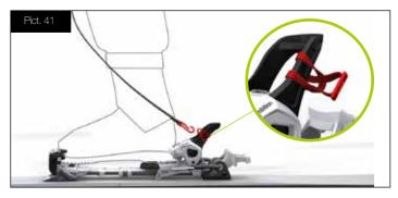
Fix the strap with the Velcro fastener on your leg and use the carabiner to connect strap and hanger again.
