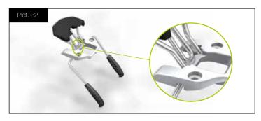
Place the brake to its position on the heel unit, push the plate to lock on binding. Fix the plate with the two screws. Ready!!!
