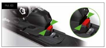
If you have too much or not enough forward pressure, check the settings and if necessary, adjust slightly at the heel and the toe. Then close the levers and check the forward pressure again. Now it should be okay.
