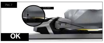
If the tester is not moveable, the gap is smaller than 0.5 mm, if you feel no resistance the gap is more than 0.5 mm. In both cases you need to re-adjust the AFD (Pict. 8).
