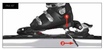
Check the elasticity and retention of the toe by pushing the boot inward and outward. The binding must recenter the boot easily and quickly from a 15 mm lateral displacement.
