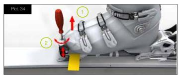
Adjust the AFS with the screw in the front so that the tester is still moveable but with a slight resistance. In this case, you reached a gap of 0.5 mm between AFS and the boot.
