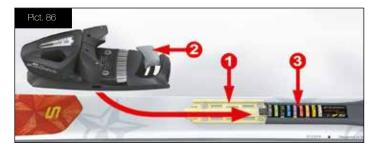
Make sure that the lever snaps in place completely ((it may be necessary to slide the toe forward and backwards slightly and to close the lever actively by hand).
