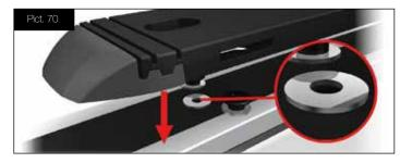
Then you can place the front and the rear part over the screws and push it in the appropriate position. Make sure that the washer stays in its position. To fix the plate, just tighten the screws.
