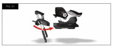
Then open the heel lever, slide the heel on the rail from the back and lock it at the appropriate boot sole marking. Don't forget to check that the lever is closed again.
