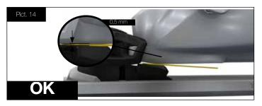
If the tester is not moveable, the gap is smaller than 0,5 mm, if you feel no resistance the gap is more than 0.5 mm. In both cases you need to re-adjust the AFD. (Pict.15)
